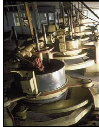
Rolling machines used in the production of black tea
